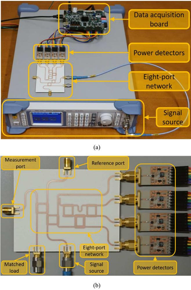
Fig. 7. Photograph of the developed eight-port reflectometer: (a) general view and (b) closer view on the eight-port network with power detectors.
