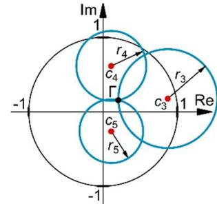
Fig. 4. Intersection of three circles indicating the measured reflection coefficient  $\Gamma$  for the arrangement of circle centers optimized for a narrow proximity of the selected point  $\Gamma_{ref}$ .
