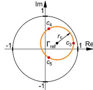
Fig. 3. Arrangement of circle centers' optimized for a narrow proximity of the selected point  $\Gamma_{ref}$ .
