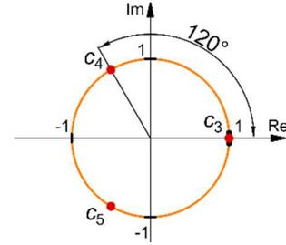
Fig. 2. Optimum arrangement of circle centers for measurement of all reflection coefficients of passive devices, for which  $|\Gamma| \leq 1$ .
