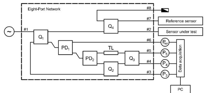
Fig. 1. A diagram of the developed eight-port reflectometer.
