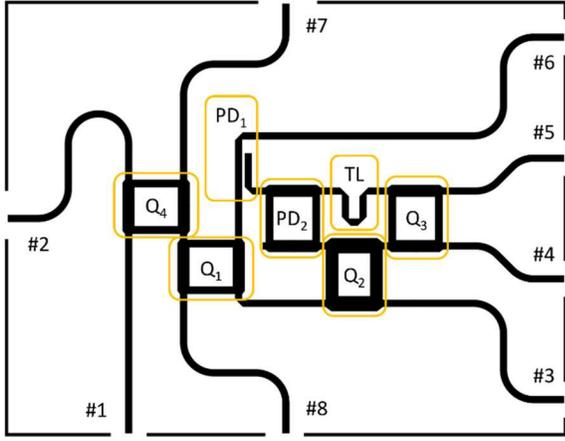
Fig. 5. Layout of the designed eight-port reflectometer.
